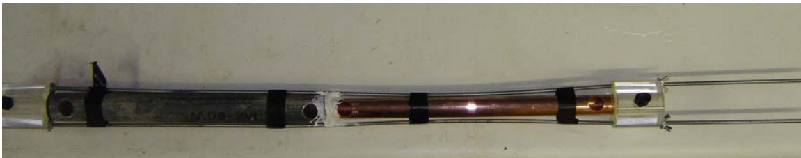
Figure 6. Photo of directly coupled LSL and copper sections used in a portion of this study
