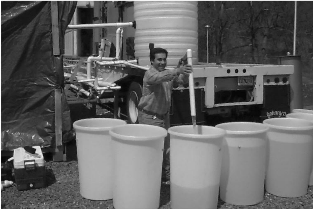
Figure 3.11 Collection of discrete samples to determine (oo)cyst time of travel through CBUD sand filtration system.
