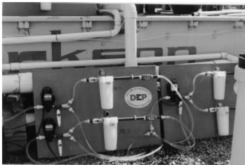
Appendix Figure 1.5 Sampling effluent with absolute pore filters.
