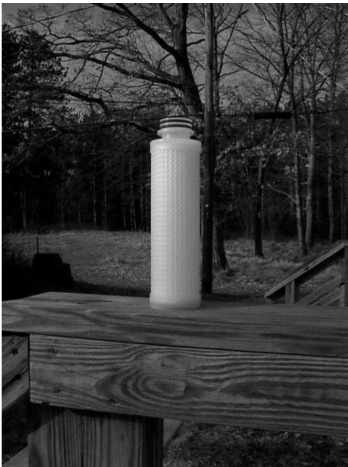
Figure 3.17 Absolute pore filter used to collect effluent samples.
