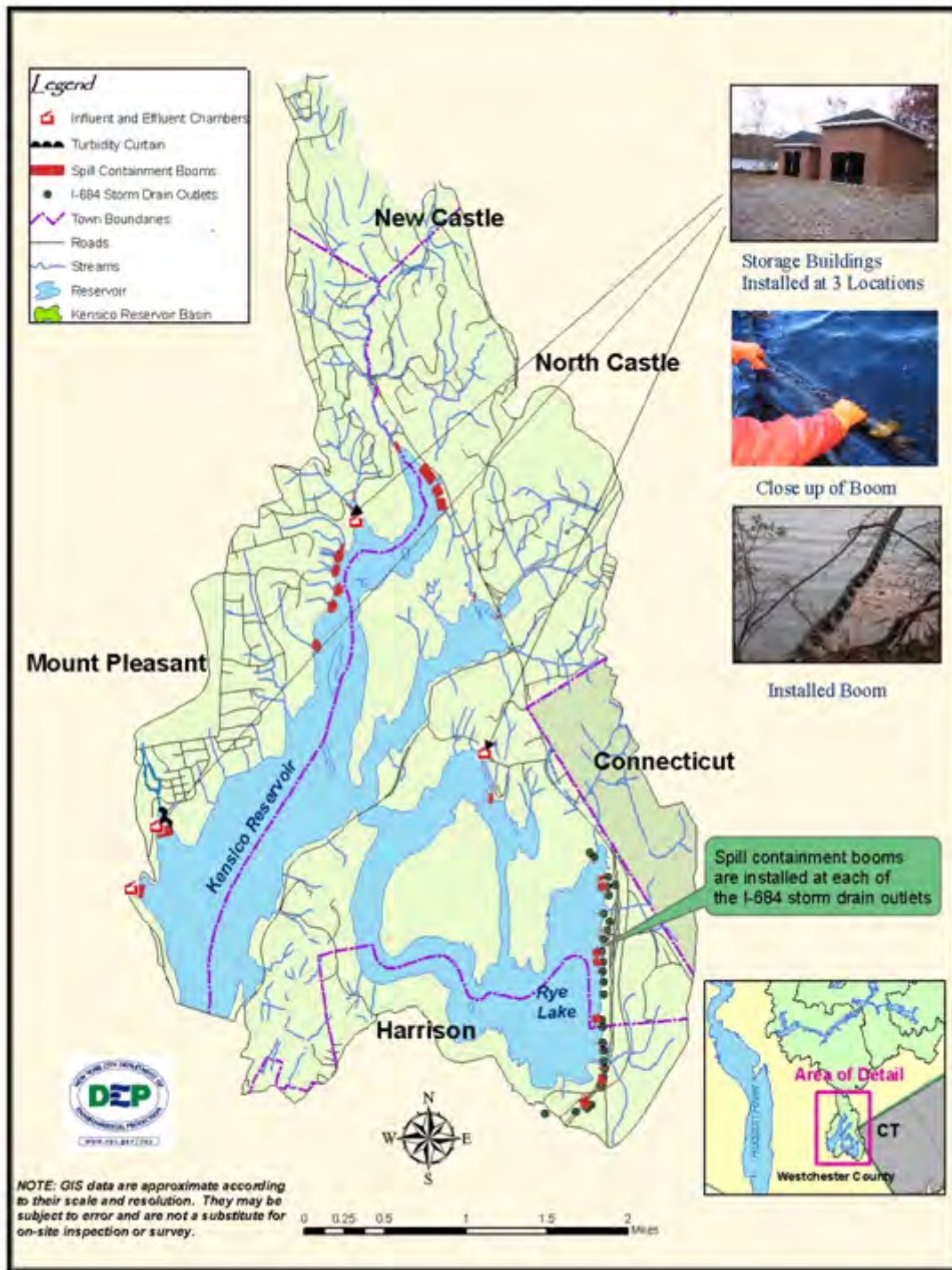
Figure 4.31 Spill containment facilities in and around Kensico Reservoir.
