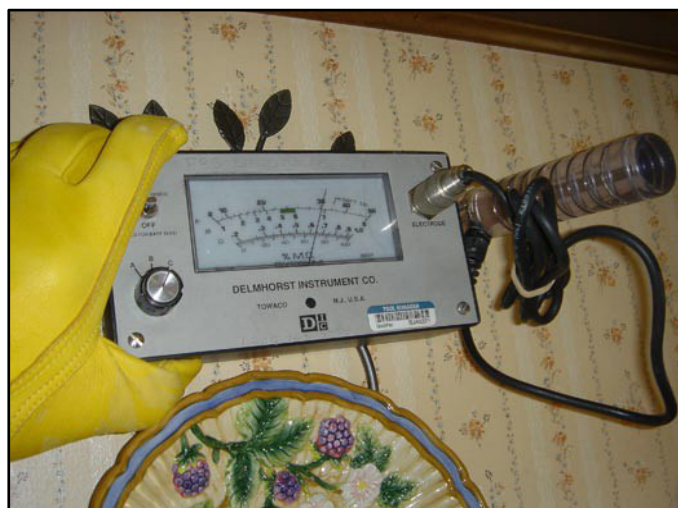
Figure 3a. An intrusive/penetrating moisture meter--recommended for final moisture readings.
