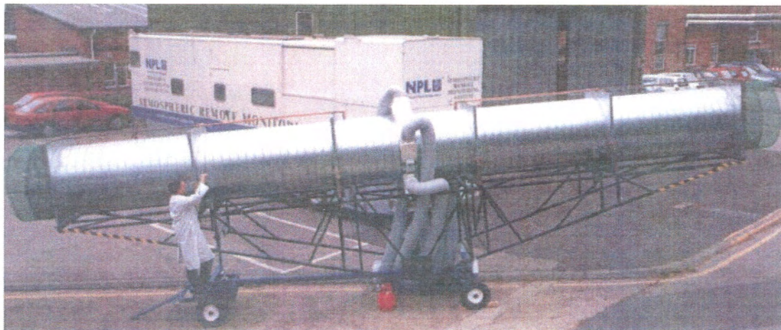
Figure A1.1 The NPL 10m calibration cell.
