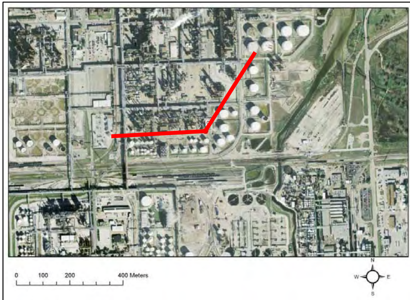
Figure 3-10. Proposed Dial Location 9: Tanks associated with benzene extraction unit and aromatics concentration unit
