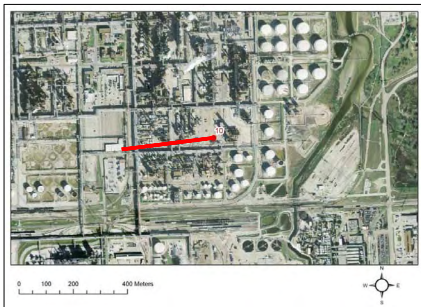
Figure 3-11. Proposed Dial Location 10: Benzene extraction unit and aromatics concentration unit fugitive emissions and tanks
