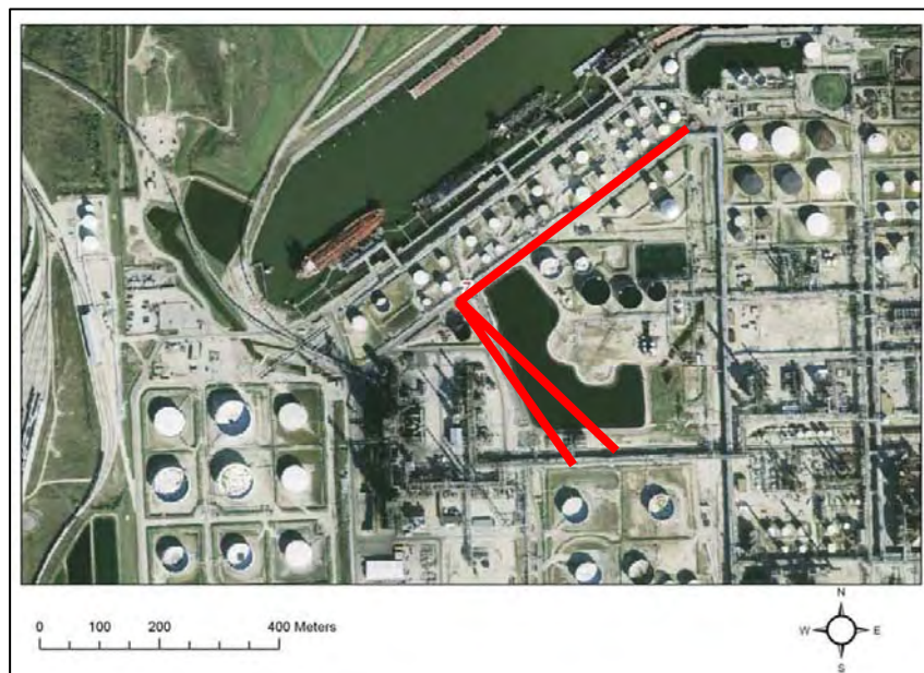
Figure 3-8. Proposed Dial Location 7: West property flare (WP FLARE), tanks east of coker units and possibly the coker flare
