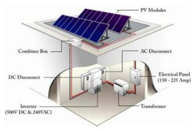
Figure 1. Major components of grid-connected PV system
