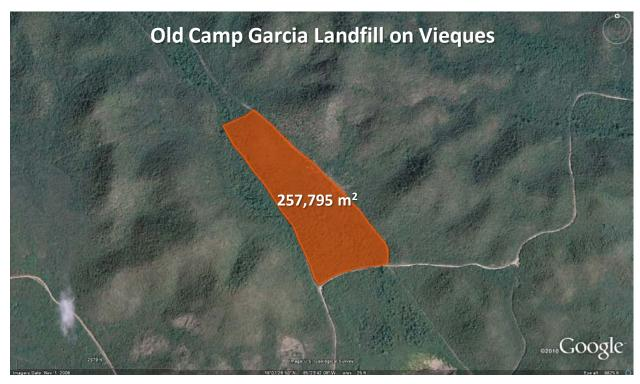
Figure 30. Aerial view of the feasible area for PV at the Old Camp Garcia Landfill on Vieques
