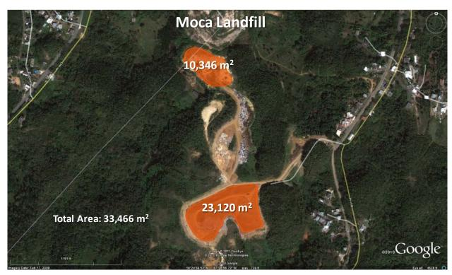
Figure 15. Aerial view of the feasible area for PV at the Moca Landfill
