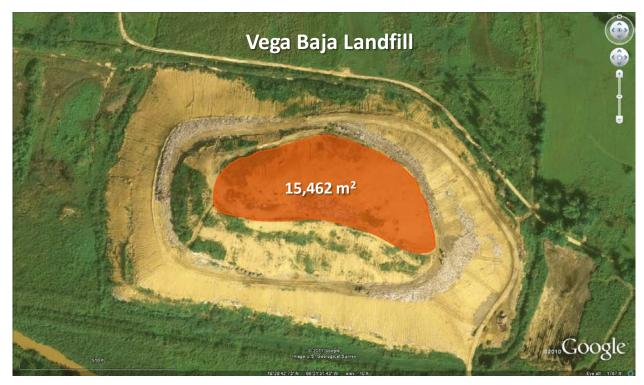
Figure 27. Aerial view of the feasible area for PV at the Vega Baja Landfill
