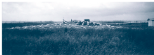
Figure 58 Test Cell – Note how pile is sagging in the center. This is due to the accelerated decomposition.
