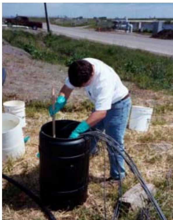
Image 6-3. Pressure transducers were tested for accuracy by submerging the sensors in water at various depths.
