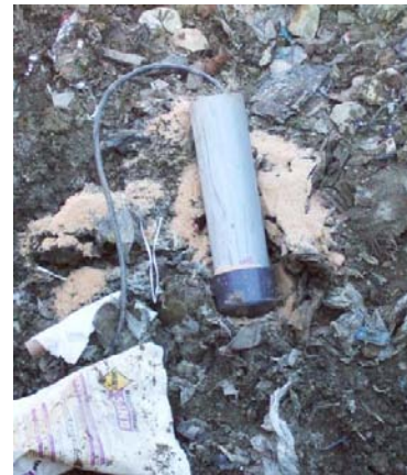
Figure 2-9 Installation of Thermocouples in Cell 6
