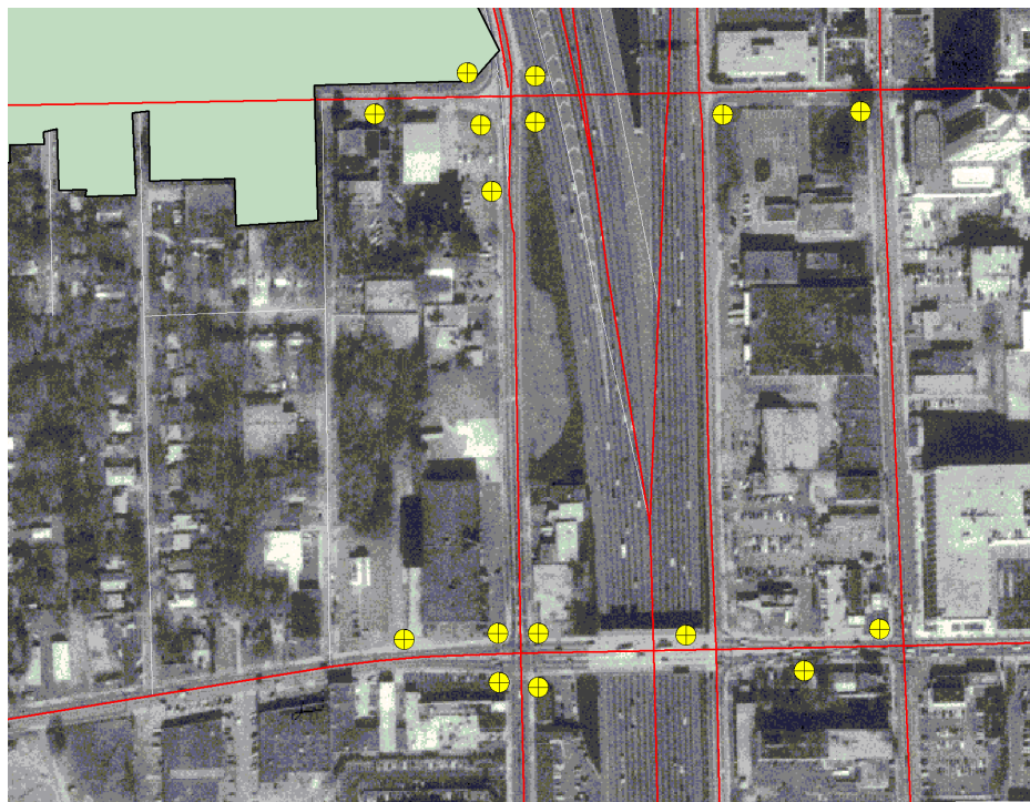
Figure 8 – Specific Receptor Locations in the Refined CALINE4 Model Run for the Year 1998 CORSIM Scenario (Maximum Predicted Concentrations did not Exceed 9.9 ppm).
