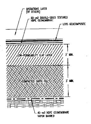
Figure 1- Typical Module D Liner Cross-section
