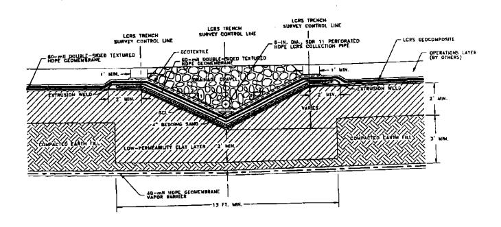
Figure 2 - Typical Module D LCRS Cross-section
