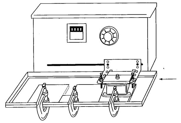
Ensure that abrasion boat rests lightly on surface by adjusting screw, if necessary.
