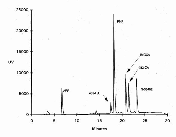
Column : Zorbax® SB-Phenyl (4.6 mm i.d. x 250 mm) Flow : 1 mL/minute Ultraviolet detection at 254 nm Gradient : 40% (0.05% H<sub>3</sub>PO<sub>4</sub> in methanol) / 60% (0.05% H<sub>3</sub>PO<sub>4</sub> in water) at 0 minutes 100% (0.05% H<sub>3</sub>PO<sub>4</sub> in methanol) at 20 minutes 100% (0.05% H<sub>3</sub>PO<sub>4</sub> in methanol) at 30 minutes
