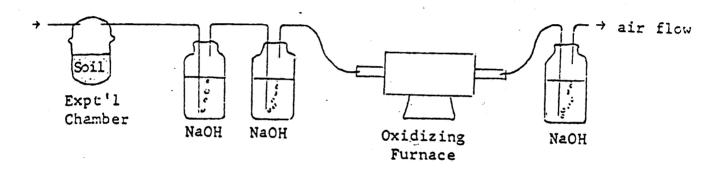
Figure  $\mathring{\mathbf{I}}$ . Aerobic soil metabolism apparatus.
