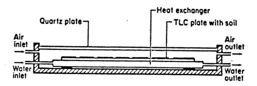
Figure 1. Photolysis apparatus.
