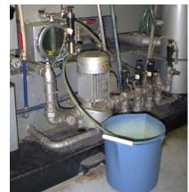
If there is potential for the vacuum water from the spotting table to contain Perc or Trichloroethene it should be managed in a wastewater treatment evaporator/atomizer or disposed of as hazardous waste. It is recommended that vacuum water from the spotting table always be managed this way due to the high potential that it could be contaminated with Perc.
