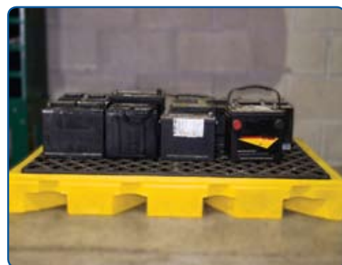
Batteries stored inside with secondary containment.
