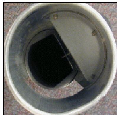
Looking Through the End of Automatic Shutoff Device
