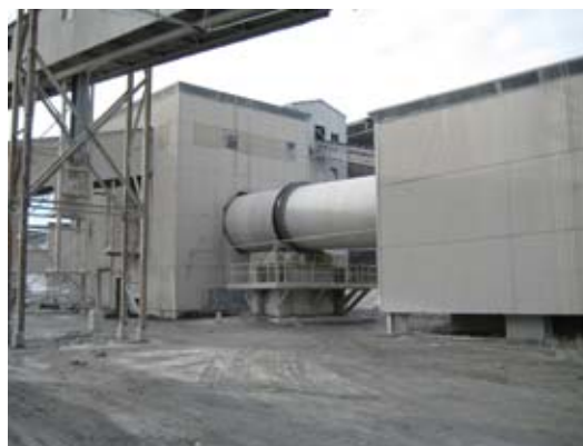
Figure 3. Machine that dries crushed and screened core sand.
