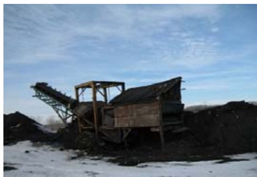
Figure 2. Machine that crushes and screens the core sand.
