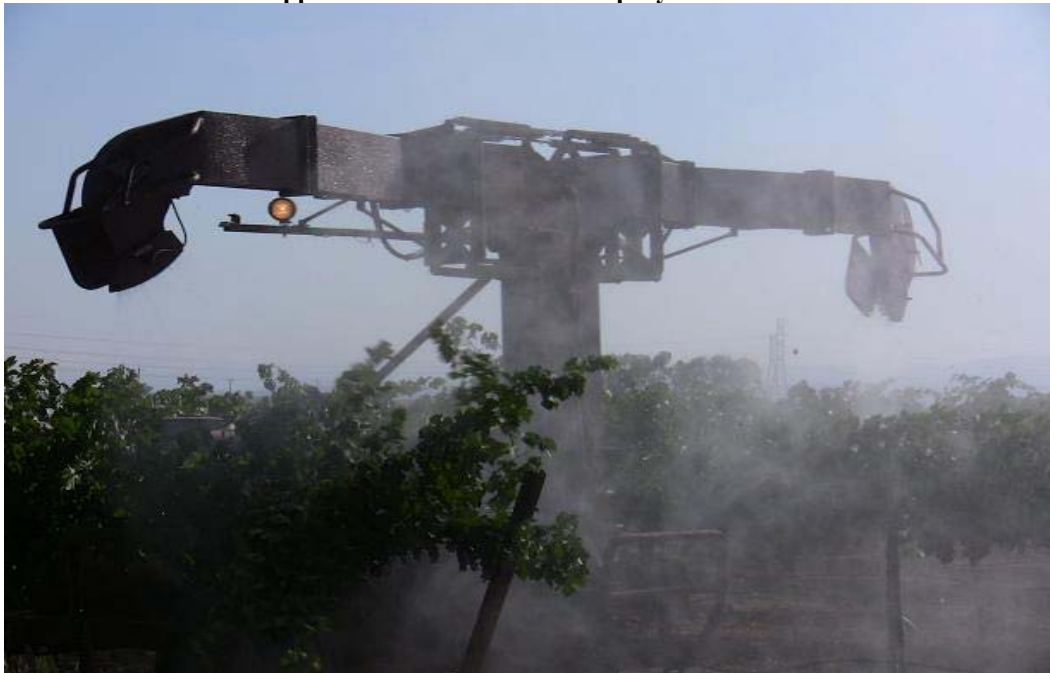
Figure 3: Closed cab airblast application with 2-row tower sprayer with electrostatic nozzles in CA grapes
