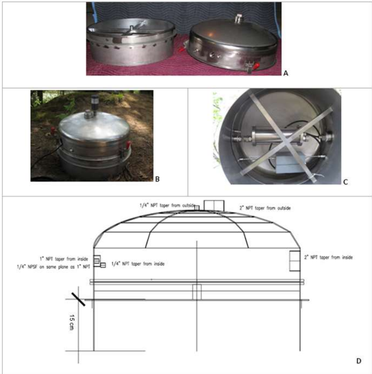
Figure 7 Flow meter Dome Chamber. (A) Photo of dome halves separated; (B) Photo of dome as it would be installed in the field; (C) Assembled unit with the flow tube and the differential pressure transducer installed inside the chamber (shown from the bottom); (D) Drawing of the dome chamber. A flange is welded around the bottom cylinder that serves as a gauge for installing the unit to a consistent depth of 15 cm.
