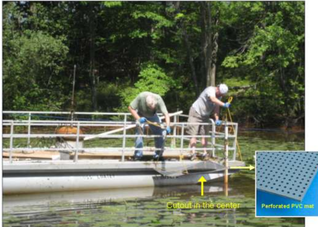
Figure 16 Placement of a perforated PVC mat prior to the flux meter installation. The perforated mat (4' x 4' in size, 1/4" thick with 1/4" hole-diameter) was placed on the sediment with a cutout in the center for the flux meter.
