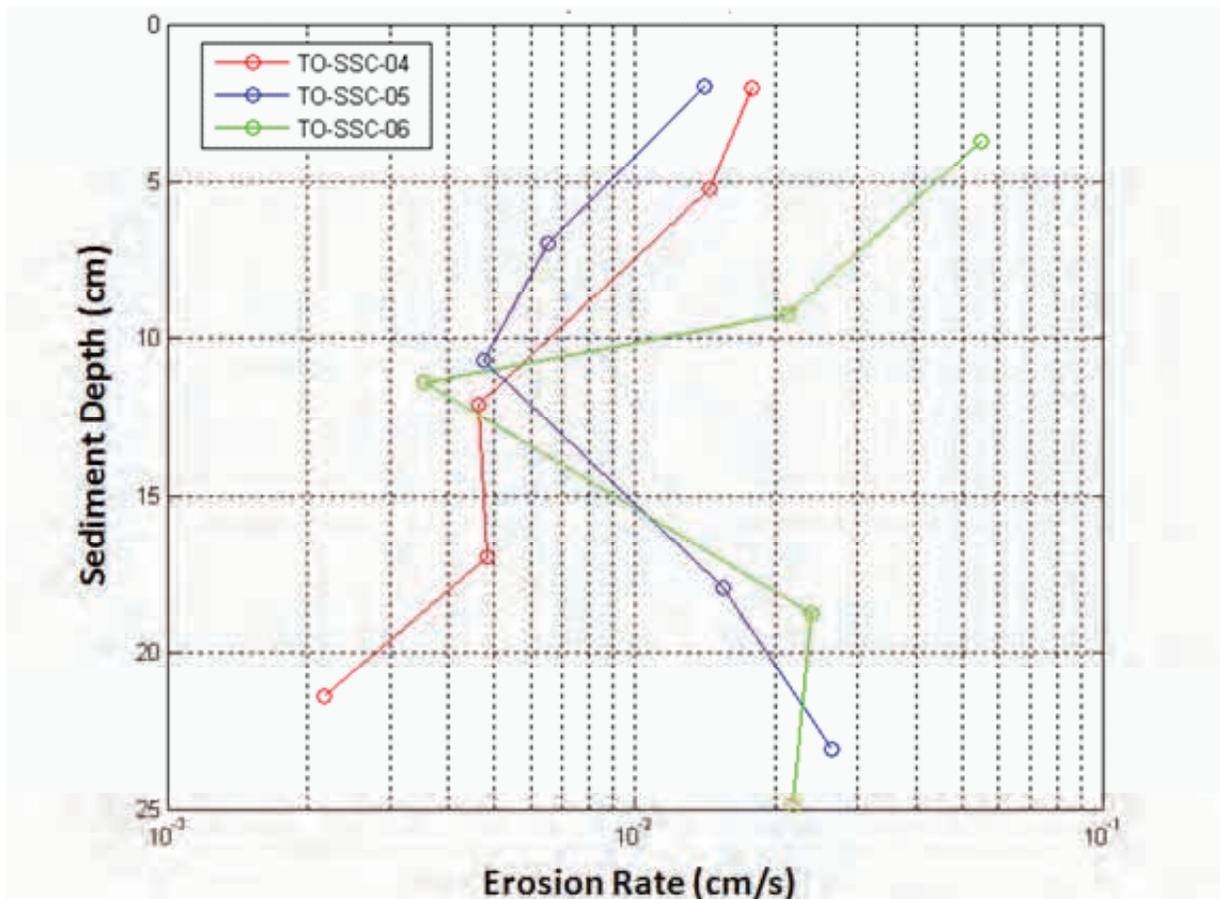
**Figure 10.** Erosion Rates (cm/s) as a Function of Depth (cm) for Three Cores on the O Transect at a Shear Stress of 1.6 N/m<sup>2</sup>.
