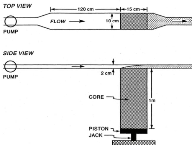
**Figure 8.** Schematic of the SedFlume Device Used to Measure Sediment Stability.
