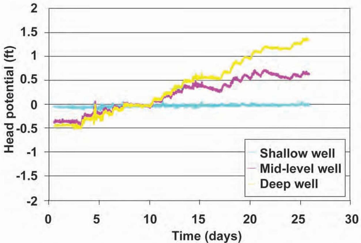
**Figure 12.** Head Potentials Shown for Vertically Stratified Wells in Lake Hartwell Sediment.
