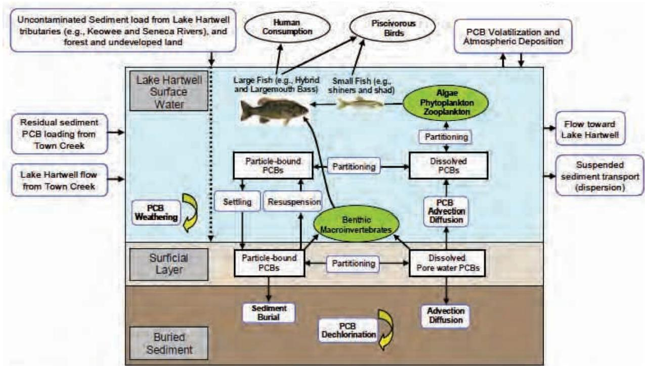
Figure 2. Conceptual Site Model for Monitored Natural Recovery as applied to Lake Hartwell (adapted from(Magar 2009).
