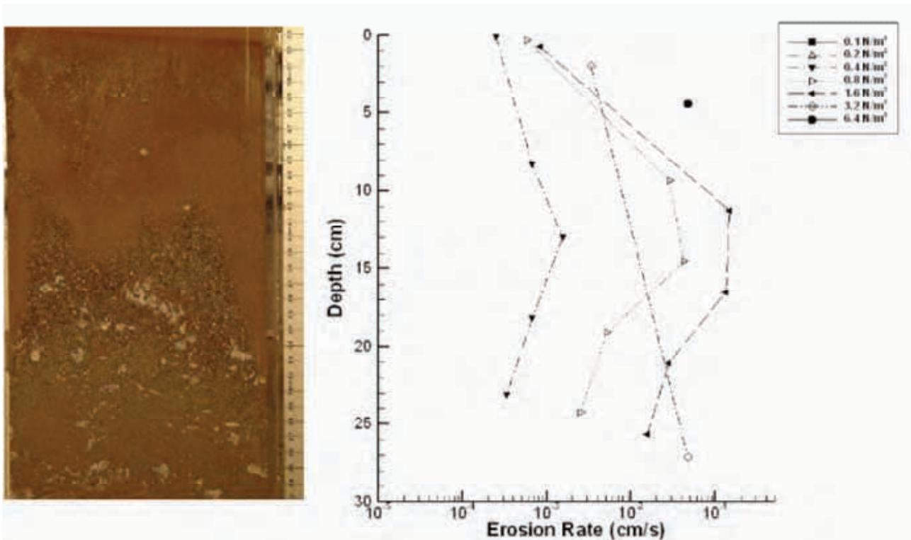
**Figure 9.** Picture of Core TN-SSE-01 Aligned with SedFlume Erosion Rate Data.
