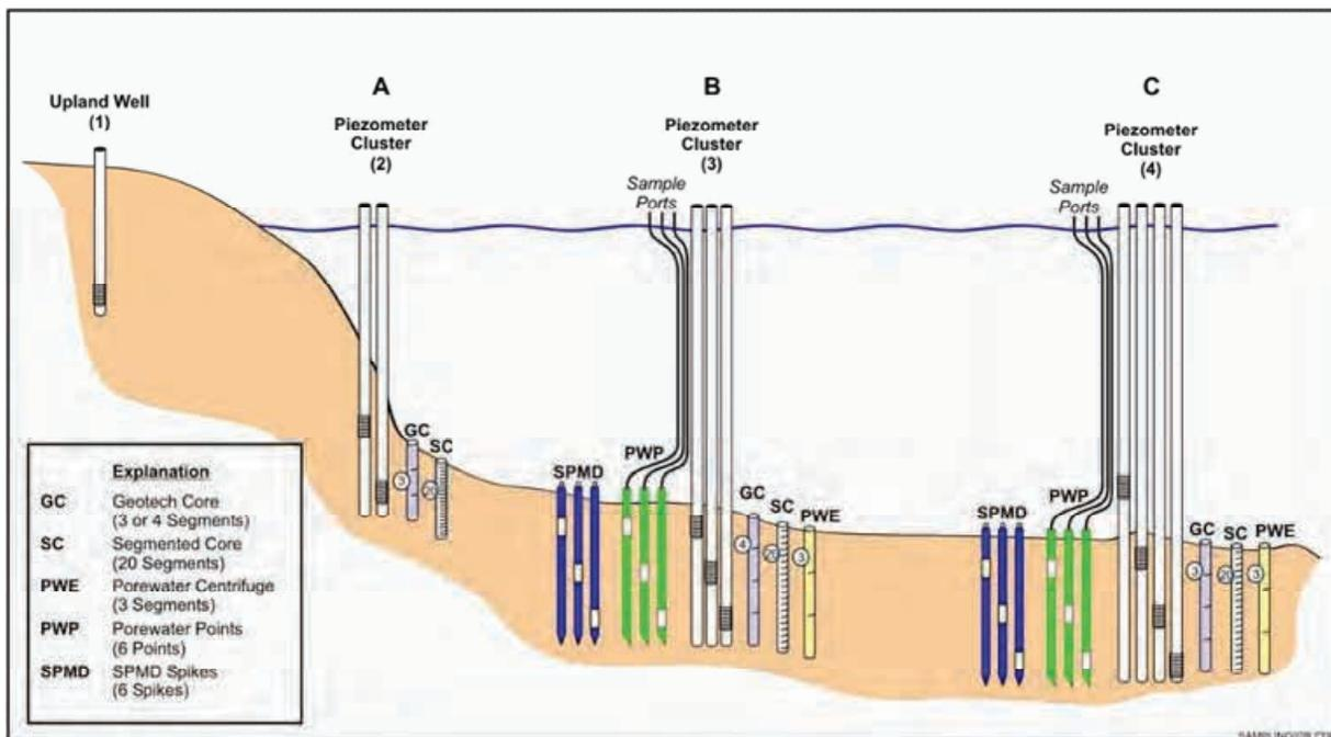
**Figure 11:** Piezometer and In Situ Sediment Deployments for Phase 4 and Phase 5
