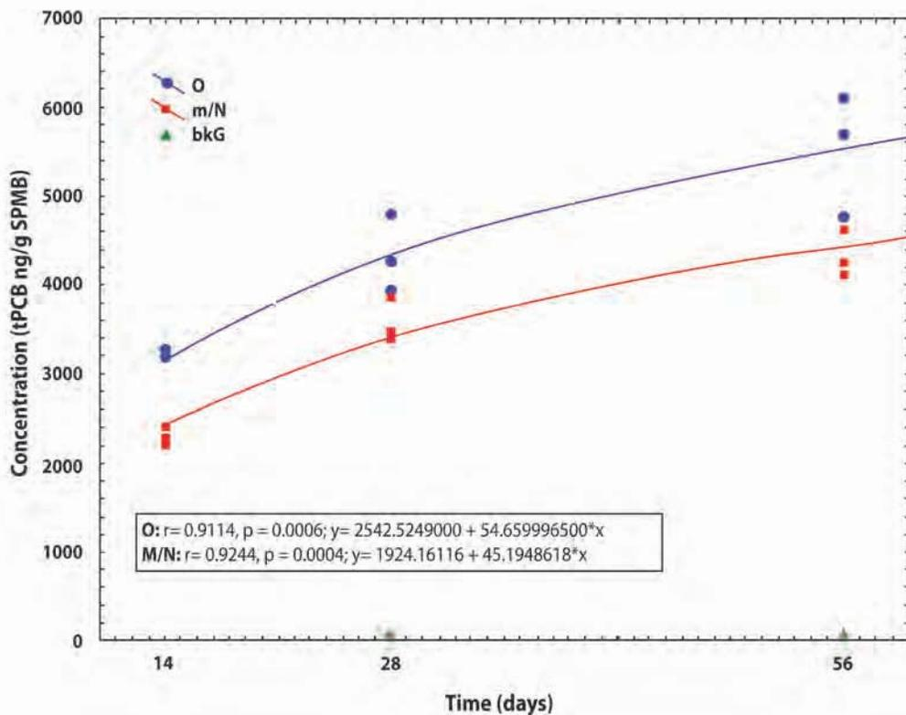
**Figure 4.** Regression Analyses (using an exponential fit) of the Time Course Experiments Comparing WCSPMDs and RSPMDs at Site T-O (top panel) and a Comparison of the RSPMDs Deployed at T-O, T-M/N, and BKG (bottom panel) (Schubauer-Berigan, 2010 - submitted).
