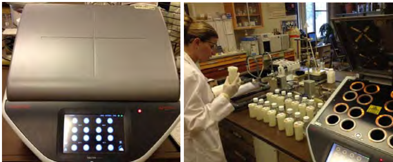
Figure 2-1. TECTA B-16 during analysis (left); Operator holding test cartridge next to TECTA B-16 ready for insertion of sample cartridges (right).
