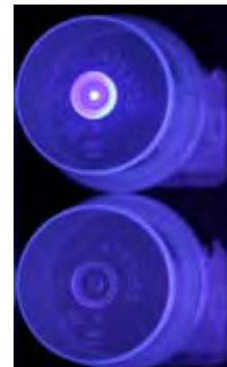
Figure 2-2. Sample cartridge exhibiting positive (top) and negative (bottom) test results.
