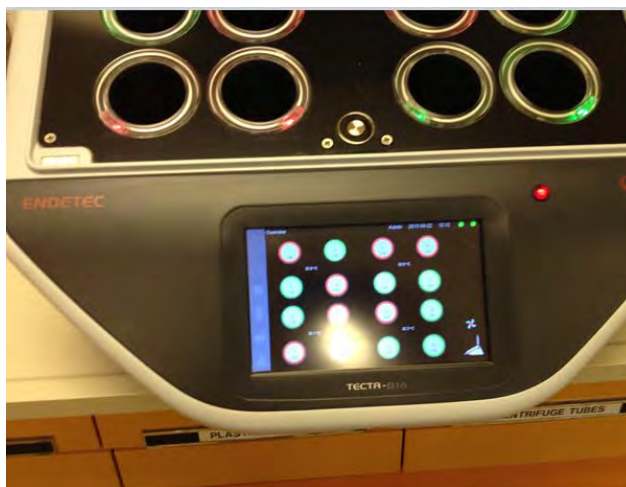
Figure 2-3. Red and green indicate results around sample chambers and on touch screen.
