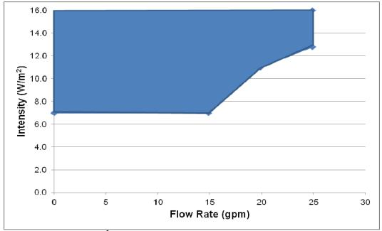
Figure 1. Set line for 40 mJ/cm<sup>2</sup> RED<sub>meas</sub> for ETS UV *Model UVL-200-4*.
