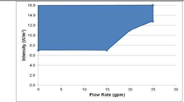
Figure 2. Set Line for Minimum 3-log and Minimum 4.0 log Cryptosporidium Inactivation for ETS UV Model UVL-200-4.
