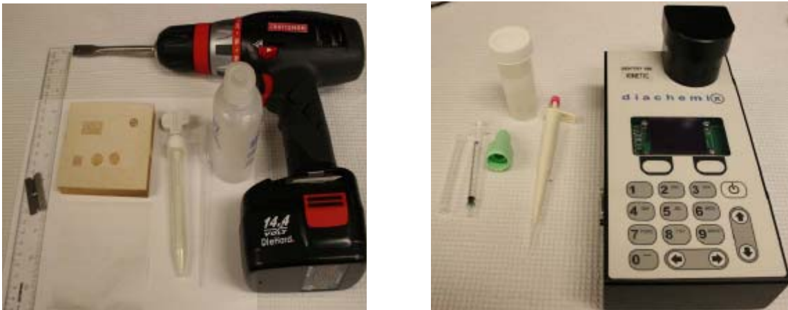
Figure 2-2. ANDalyze Lead-in-Paint Test Kit Test extraction kit (left) and testing kit (right)
