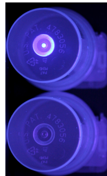
Figure 2-2. Positive (top) and negative (bottom) test results
