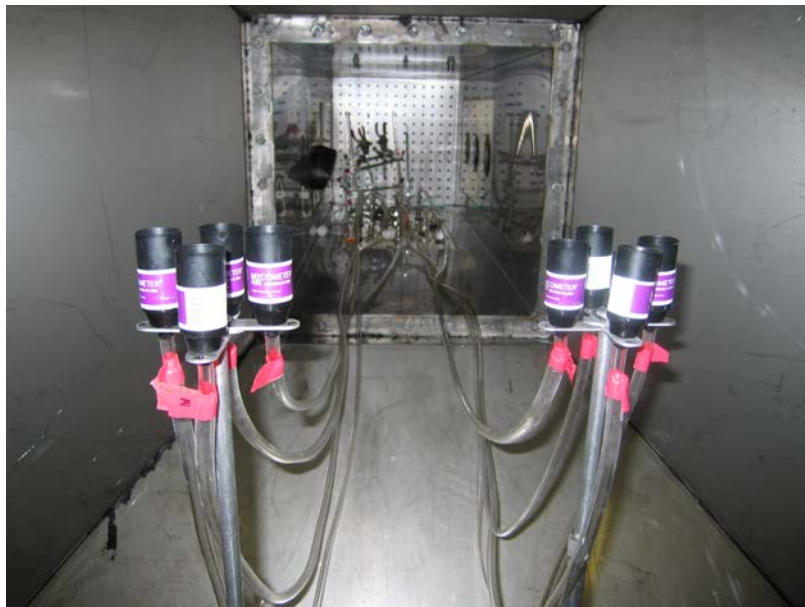
Figure 3-2. Sampling Cartridges Inside the ARCA Chamber with Tubing Leading to Pumps Outside the ARCA Chamber
