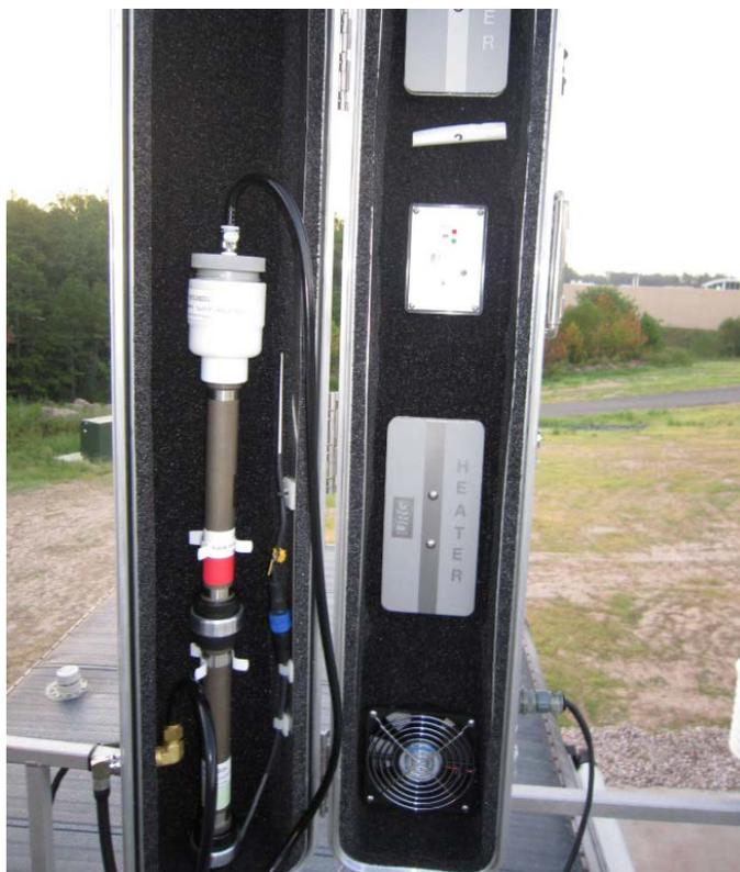
**Figure 3-3. Installed denuder/filter pack sampling train.**
