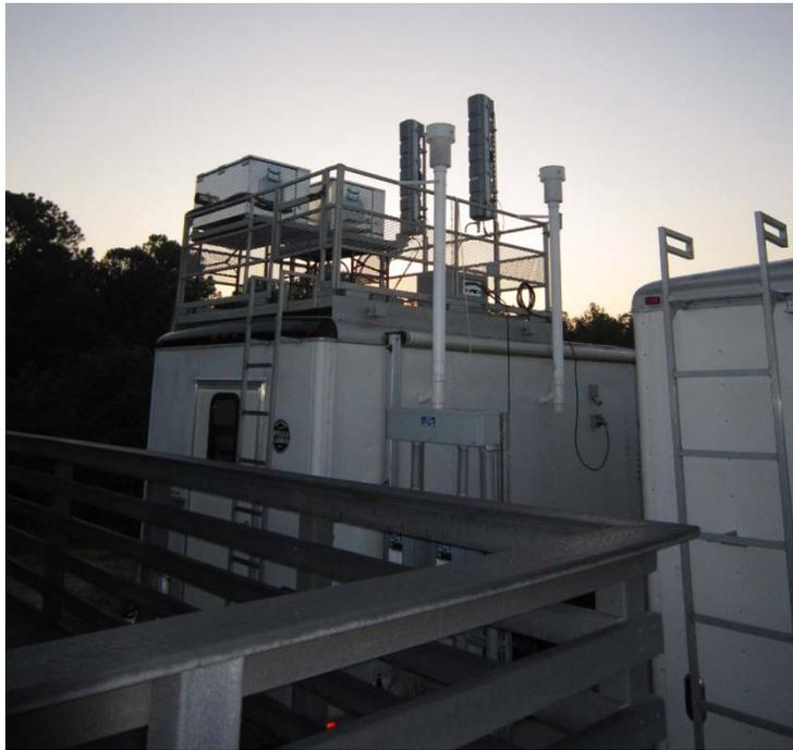
**Figure 3-1. Sampling trailer with denuder/filter pack samplers.**
