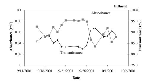
Figure 4-5. Laboratory UV Absorbance and Transmittance for Feed and Effluent Water
