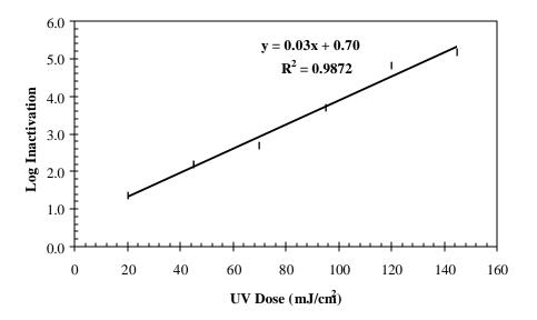
Figure 4-1. Dose Response Curve for Preliminary Collimated Beam Test (9/5/01)
