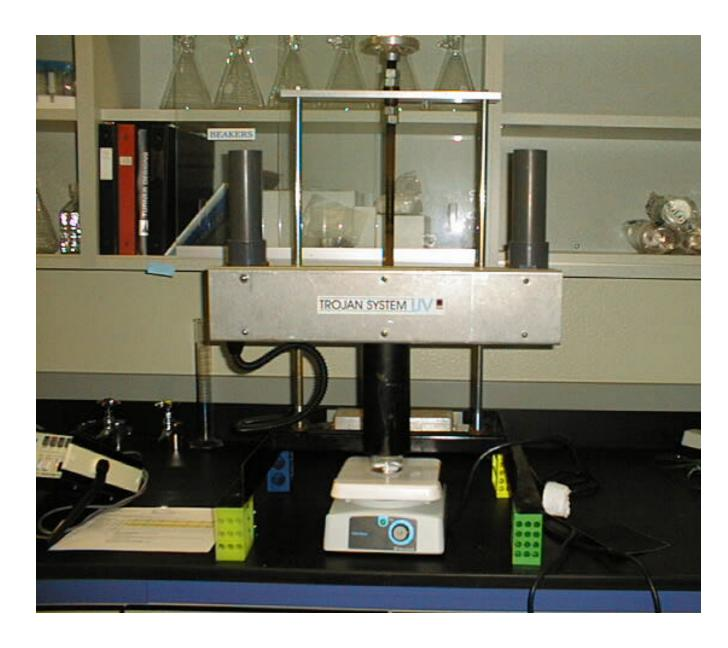
Figure 3-1. Photograph of Collimated Beam Unit
