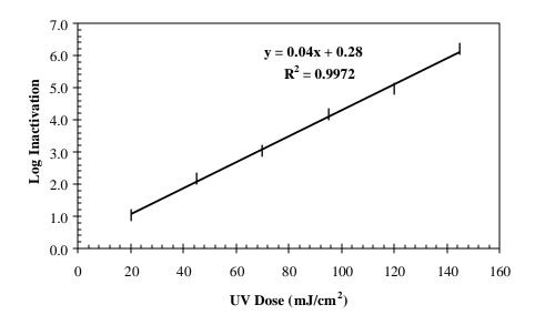
Figure 4-6. Dose response Curve from Collimated Beam Testing (9/14/01)
