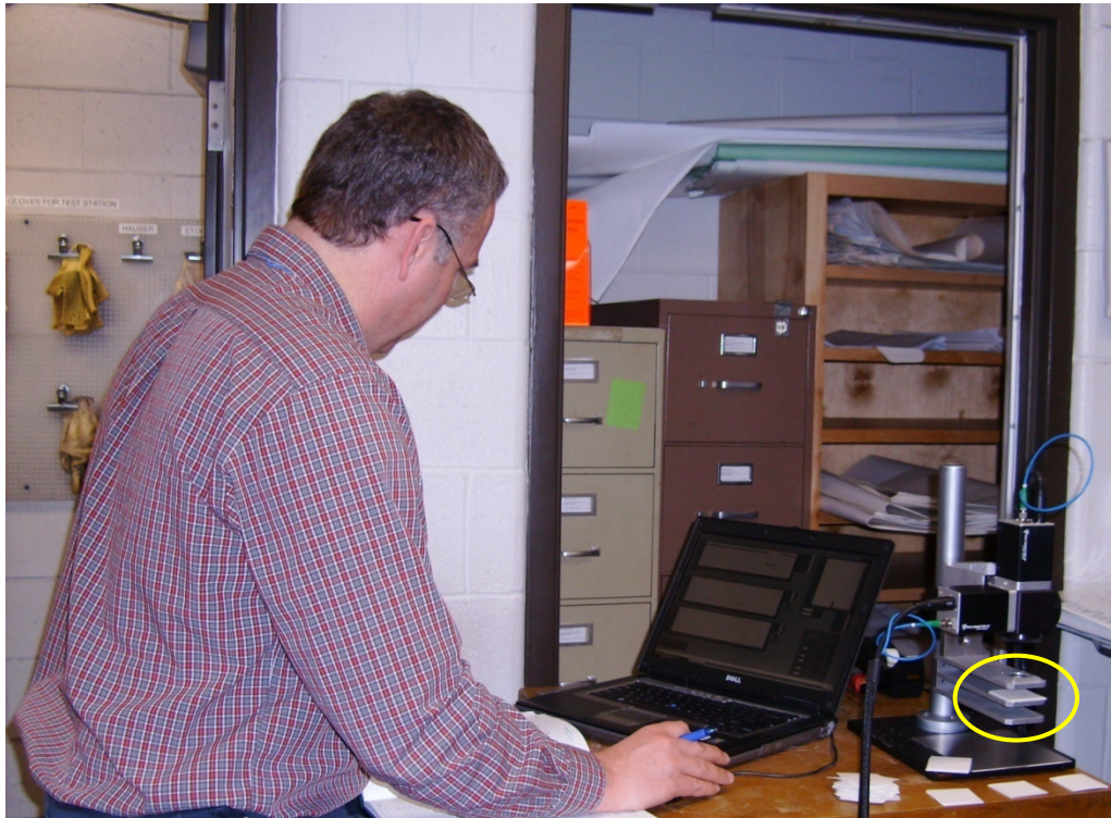
Figure 3-6. THz sensor system in the Laboratory. One stack of mid-weight paper is seen in the sample holder (highlighted in a yellow oval).
