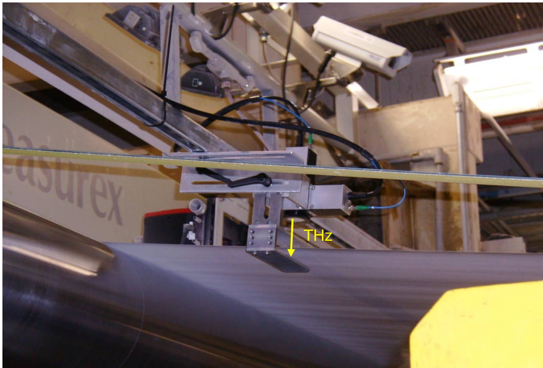
Figure 3-3. Close-up of THz Sensor in the Production Line. The paper on the production line is seen between the two lower plates of the gauge. The yellow arrow indicates the THz photon path.
