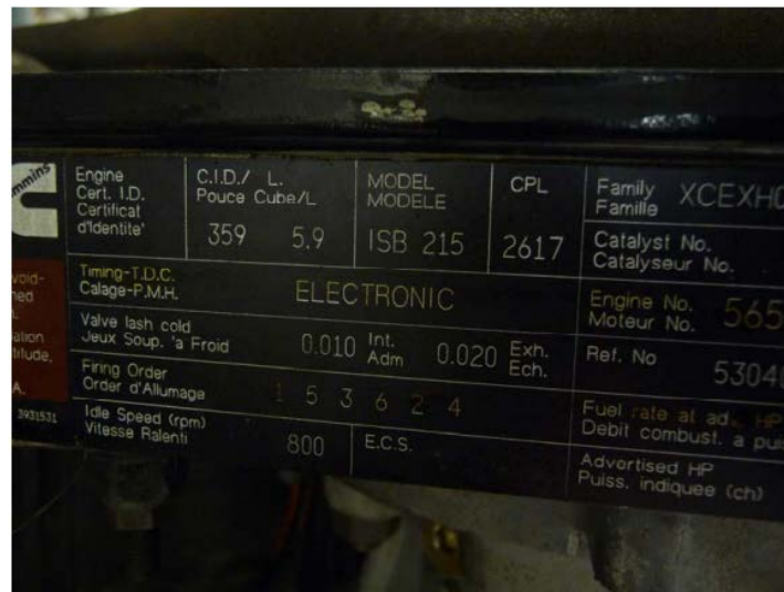
Figure 2. Identification label for 1999 Cummins ISB 215 showing engine model.
