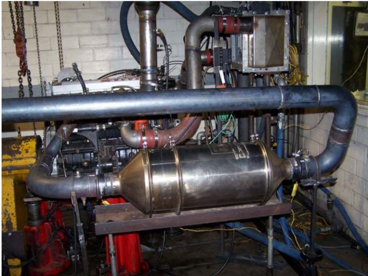
Figure 1. The Baumot BA-B system installed for emissions tests.
