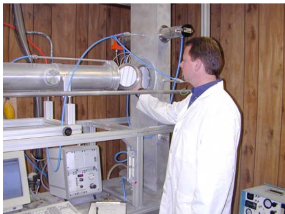
Figure 2: Installing a Fabric Sample in the Test Apparatus for the Baghouse Filtration Products
