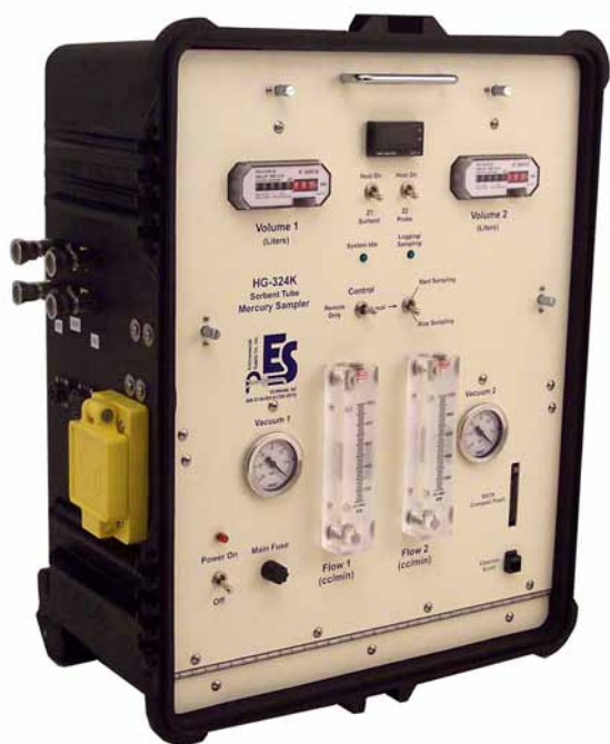
Figure 2-1. HG-324K Sorbent Tube Mercury Sampling System
