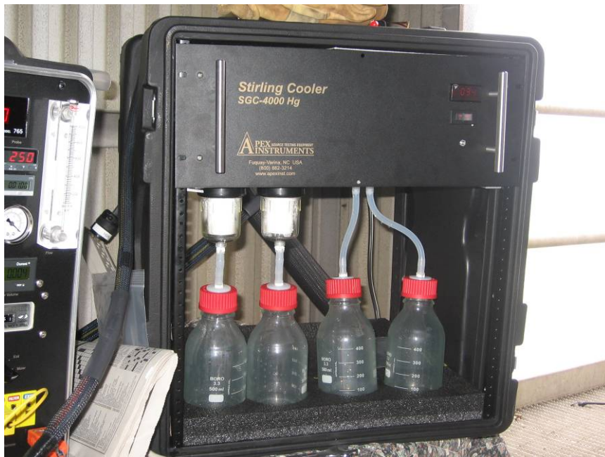
Figure 2-2. Apex SGC 4000 Hg Stirling Gas Conditioner
