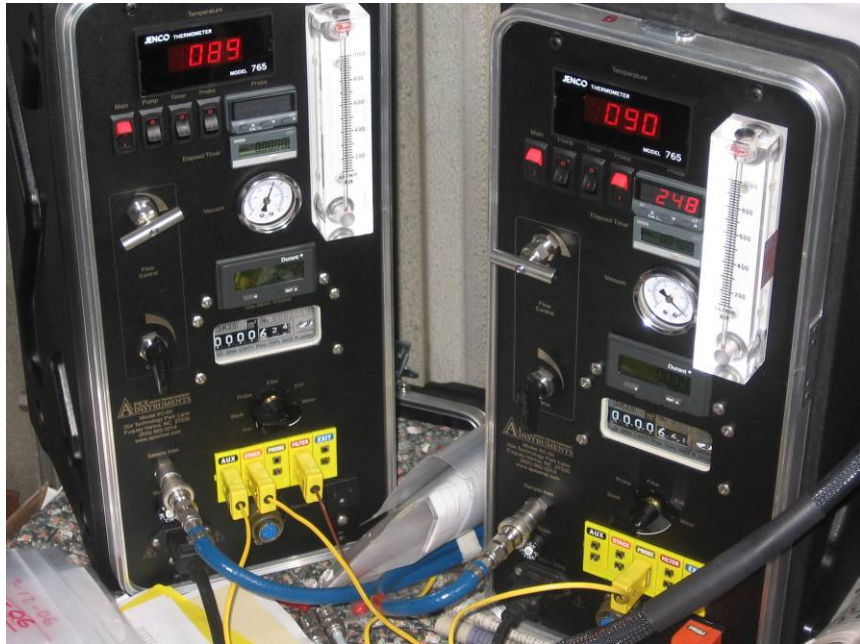
Figure 2-1. Apex XC-60 Gas Sampling Consoles
