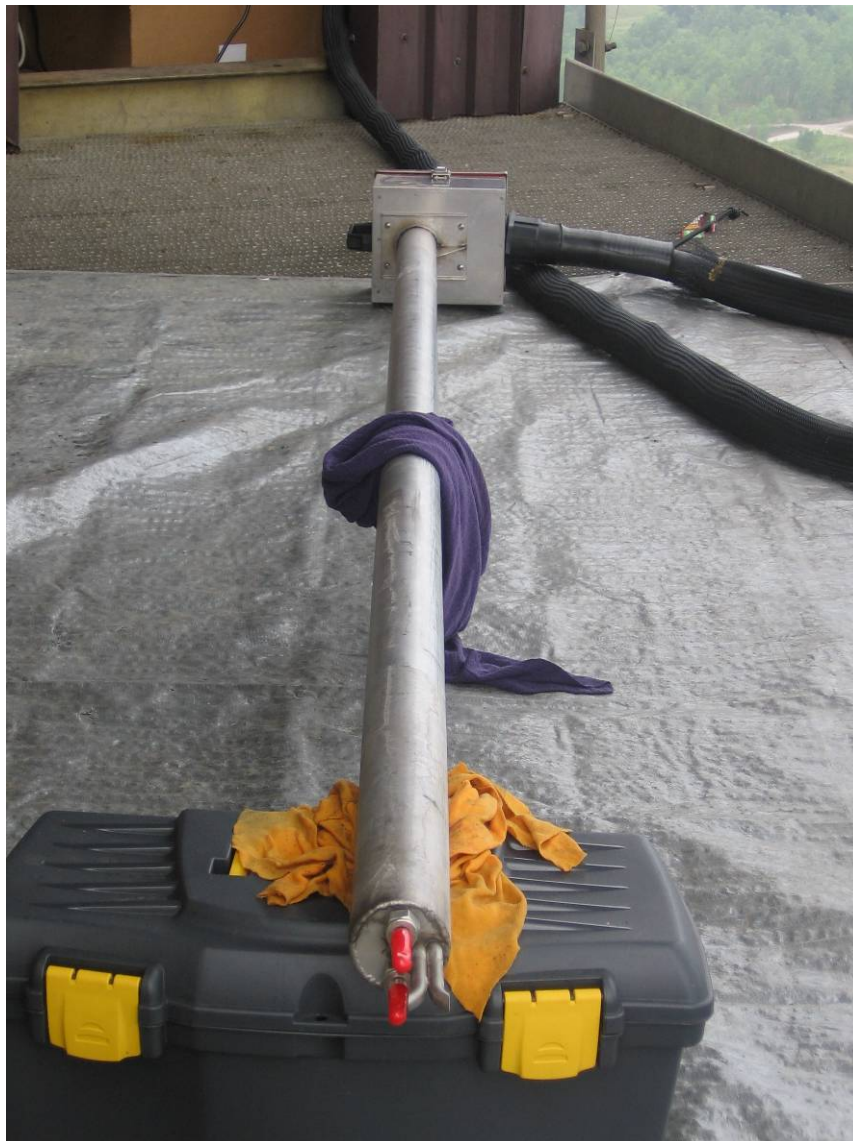
Figure 2-3. Apex Dual Trap Sampling Probe and Heated Line
