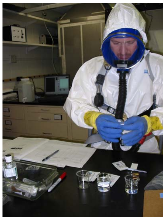
Figure 6-2. Testing of Eclox™-Pesticide Strips with the Non-Technical Operator Wearing PPE
