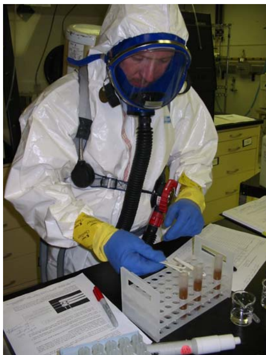
Figure 6-2. Testing of the OP-Stick Sensor with the Non-Technical Operator Wearing PPE
