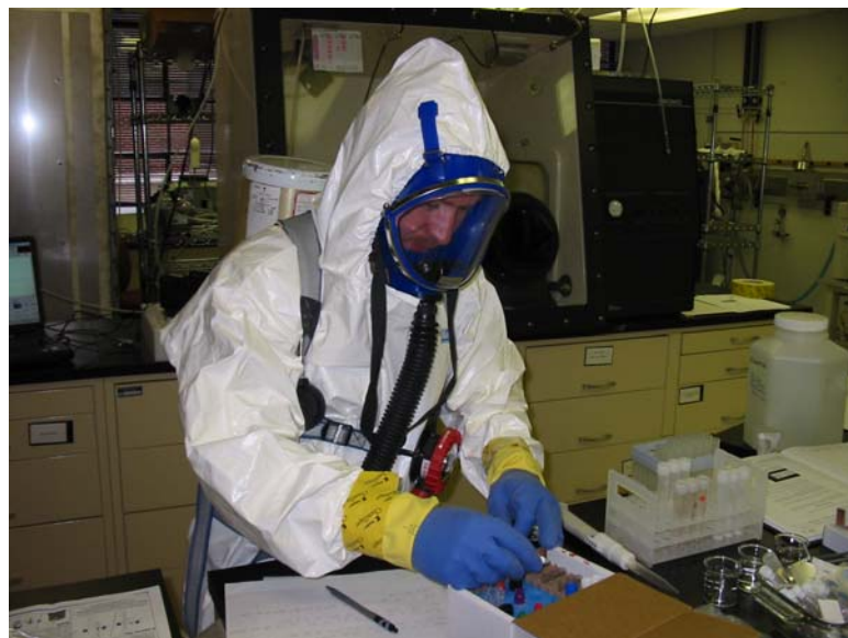
Figure 6-2. Testing of the OP/C Screen Kit with the Non-Technical Operator Wearing PPE
