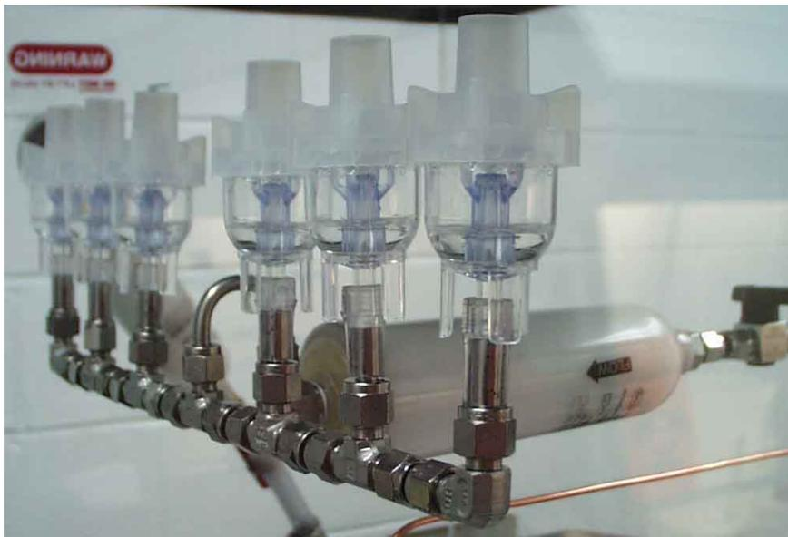
**Figure 3-4. Nebulizers in the Plas-Labs Compact Glove Box**
