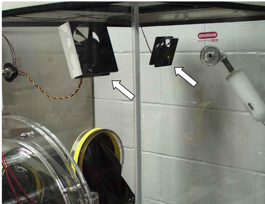
**Figure 3-3. Fans in the Plas-Labs Compact Glove Box**
