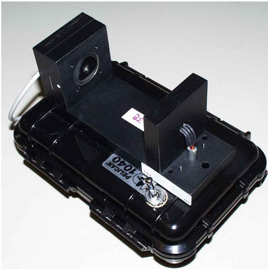
**Figure 3-5. SAIC Chlorine Dioxide Monitor**
