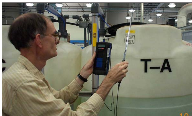
Photo 13. Sampling air over acid tank porthole for HC1.
