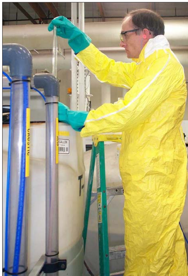
Photo 11. Extracting acid tank sample with glass Coliwasa tube.
