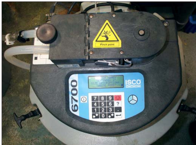
Photo 6. Automatic ISCO Sampler, top view with tube entering pump and keypad for programming the sampling outline.
