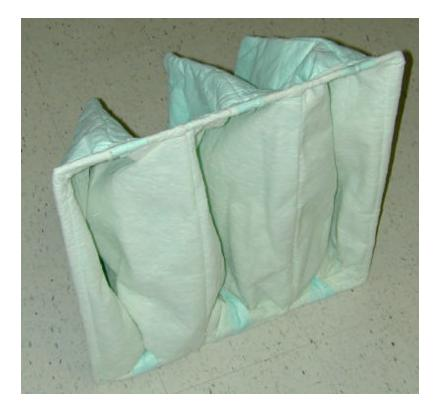
Figure 1. Photograph of the Koch Duo-Pak 650 paint overspray arrestor.
