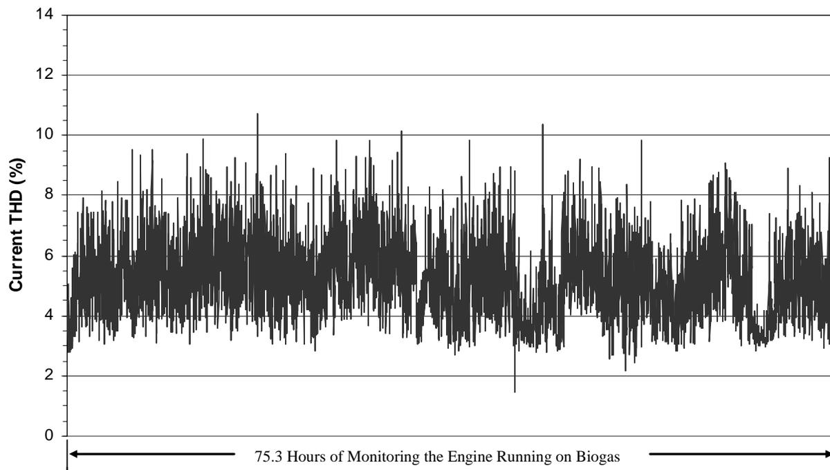
Figure 2-8. IC Engine Current THD During Extended Test Period
