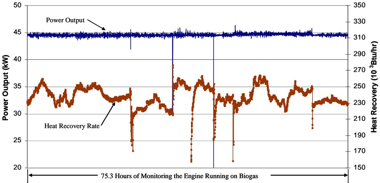
**Figure 2-3. Heat and Power Production During the Extended Monitoring Period**
