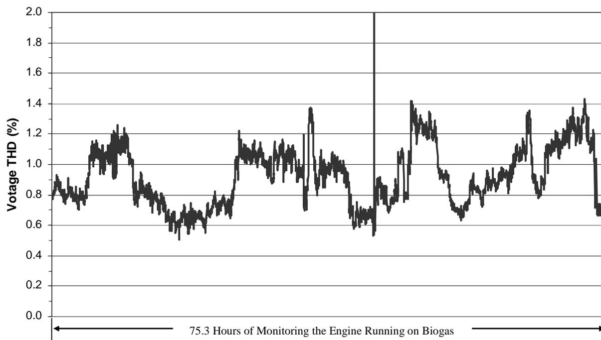
Figure 2-9. IC Engine Voltage THD During Extended Test Period
