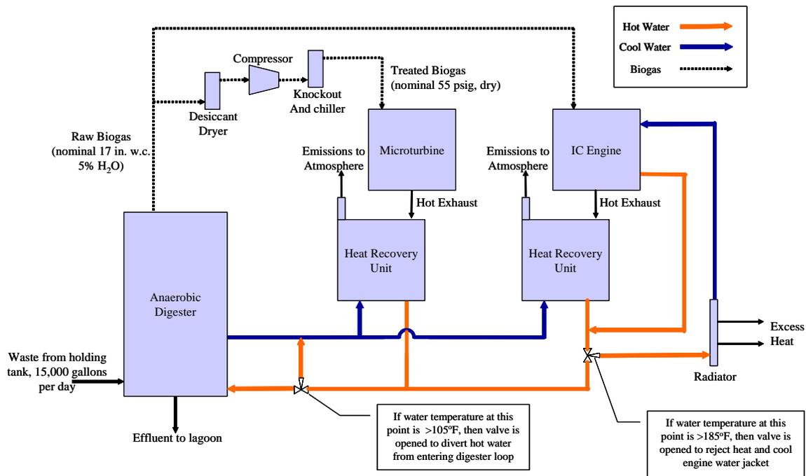
**Figure 1-4. Colorado Pork Waste-to-Energy Process Diagram**
