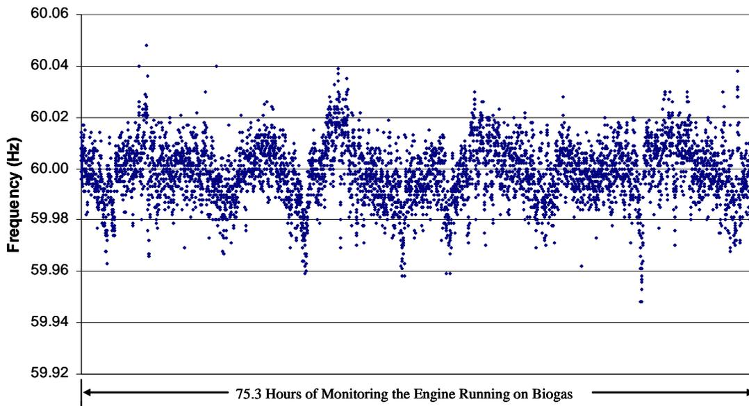
**Figure 2-5. IC Engine Frequency During Extended Test Period**
