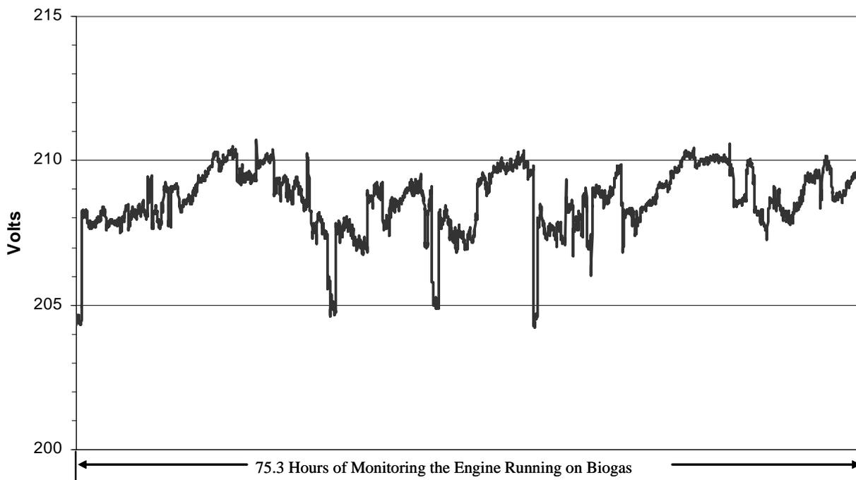
**Figure 2-6. IC Engine Voltage During Extended Test Period**
