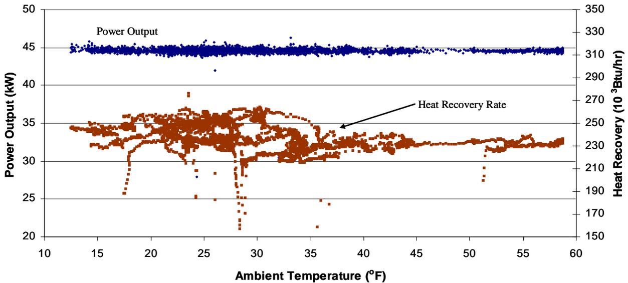
**Figure 2-4. Ambient Temperature Effects on Power and Heat Production**
