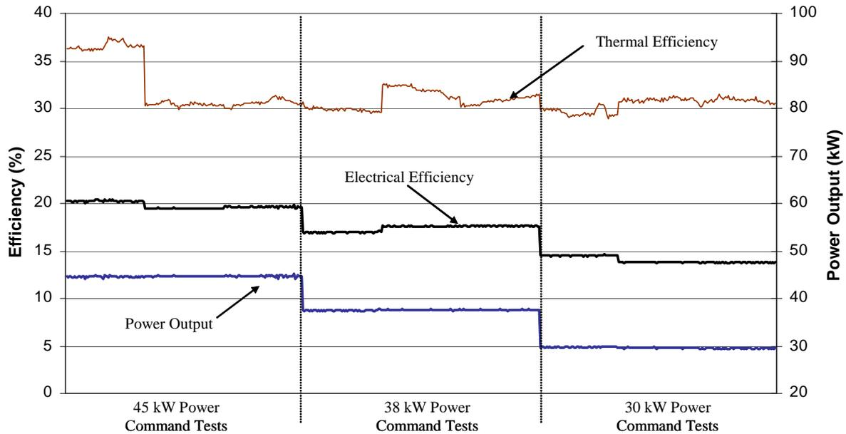
**Figure 2-2. CHP System Efficiency During Controlled Test Periods**
