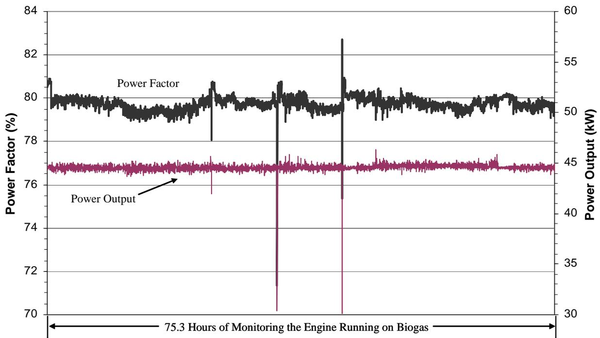
Figure 2-7. IC Engine Power Factor During Extended Test Period
