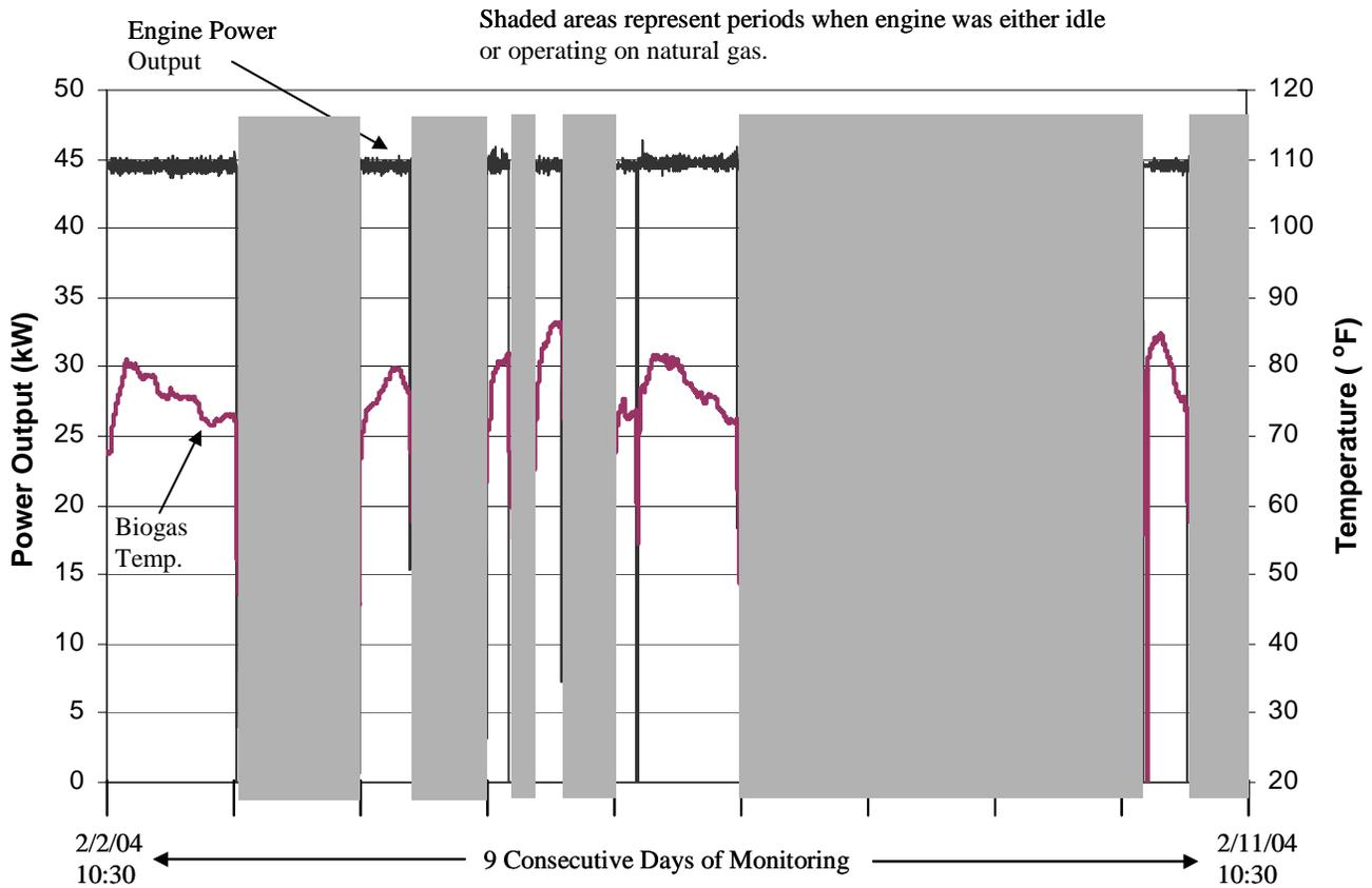
**Figure 2-1. Engine Operations During the Extended Monitoring Period**
