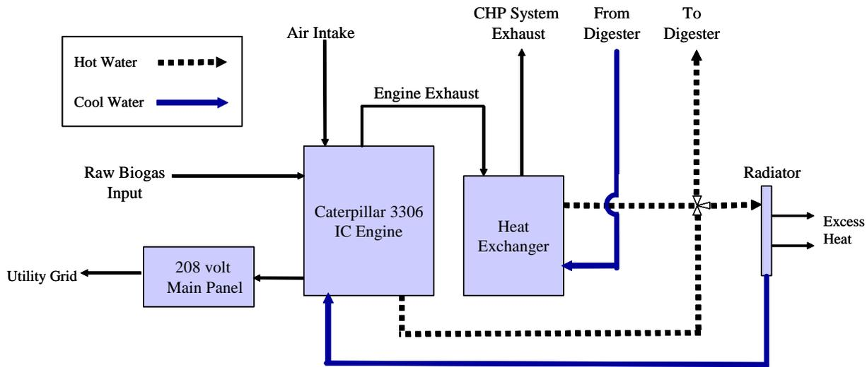
Figure 1-2. IC Engine CHP System Process Diagram
