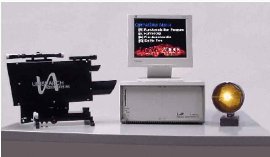
Figure 2-1. UNISEARCH Associates LasIR TDL Open-Path Monitor, Controller, Telescope, and Retroreflector
