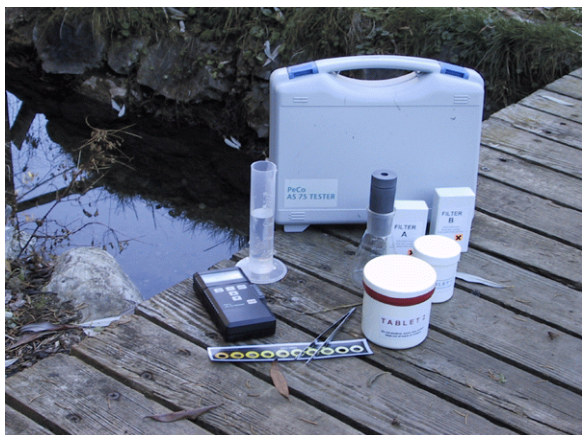
Figure 2-1. Peters Engineering AS 75 Arsenic Test Kit
