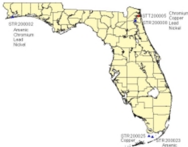
Figure 2-5: State scale stations with one or more metals exceeding TEL limits, IMAP Sampling summer 2000. Metals listed near each station are those for which concentrations exceeded the TEL. Site STR200008 also exceeded the TEL for mercury. See text for additional explanation.
