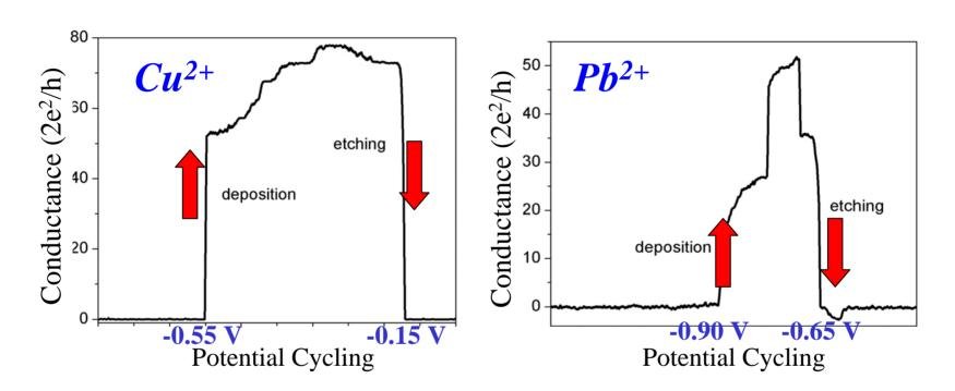
➤ Different metals have different deposition & stripping potentials.
