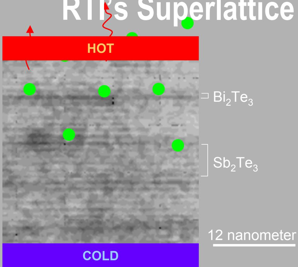
The RTI breakthrough arises from reducing heat transmission without disrupting electron flow
