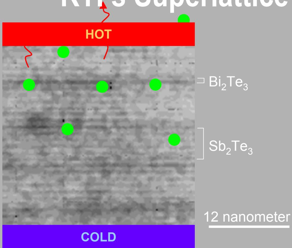
The RTI breakthrough arises from reducing heat transmission without disrupting electron flow
