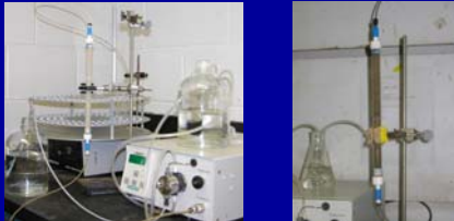
(a) Column setup for in-situ TCE degradation; (b) A close-up of the column as Fe/Pd nanoparticle suspension was introduced.
