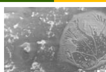
1.2 wt % HMW Chitosan + 1.5 wt % Urea in 90 % Acetic Acid Solution Air Flowrate 25 ft 3 /hr Air Temperature 70 °C
