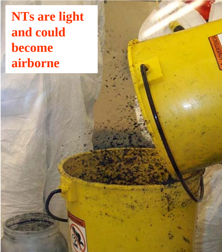
Pouring HiPco-NT between Containers at Rice Facility (Courtesy of Drs. Maynard & Baron, NIOSH)
