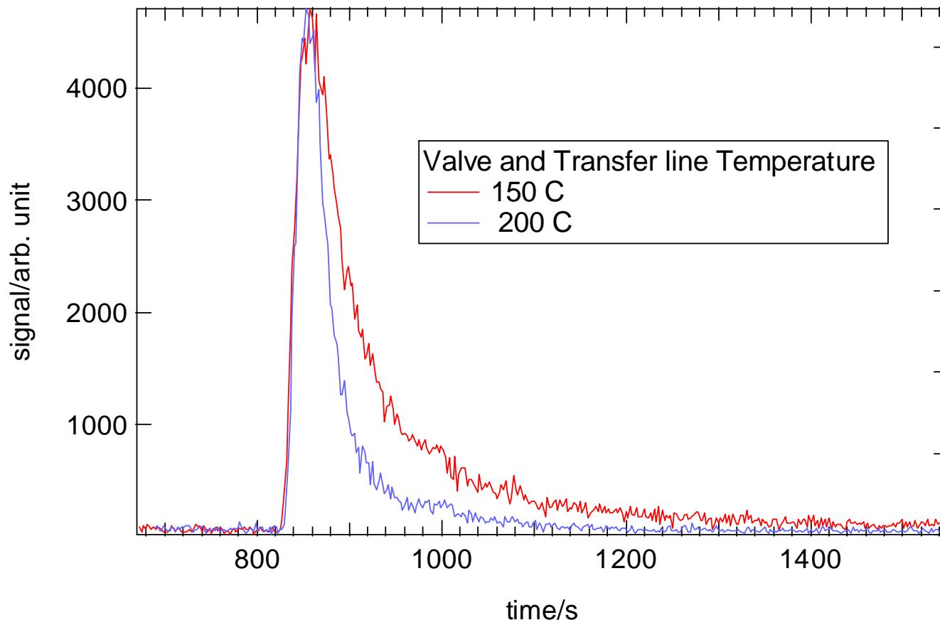
Higher transfer line and valve temperatures improve transfer times...*coatings are important.*
