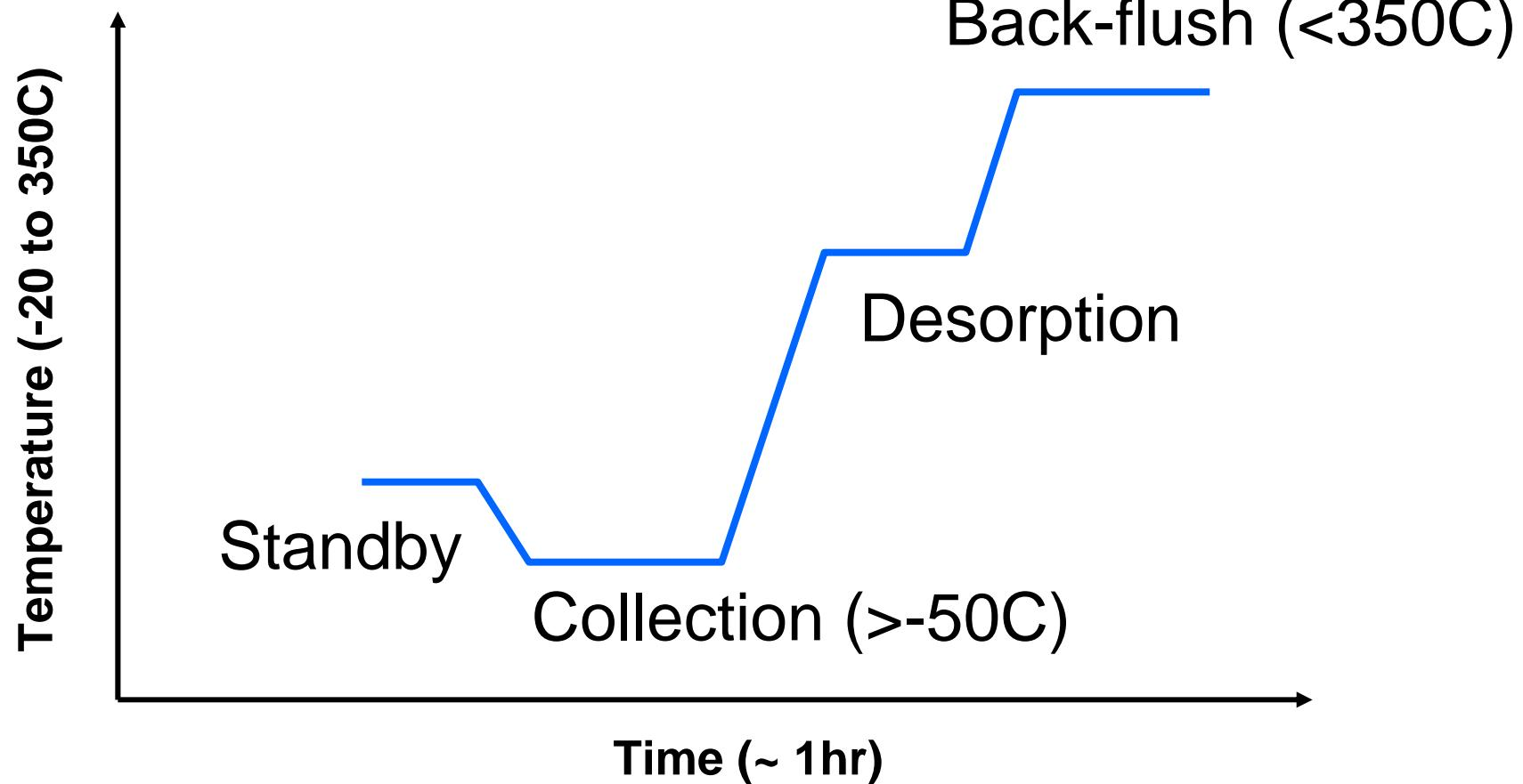
*Automated cycle controlled by microcomputer*
